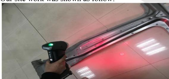
Figure 1: Using Handy Scan 700 to scan a drawn part.
