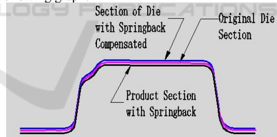
Figure 6: Die profile reconstructed with Springback compensation by CATIA software.
