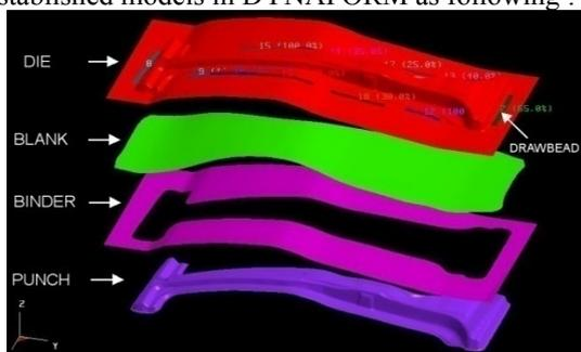
Figure 7: Dynaform simulation models.
