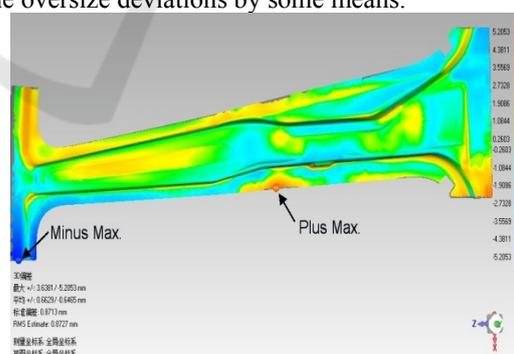
Figure 3: Springback value contour.
