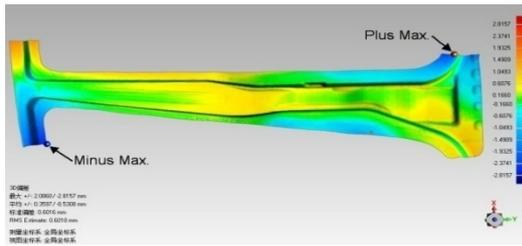
Figure 9: Springback of a B pillar stamped by an improved die.
