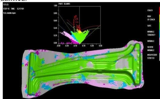
Figure 8: FLD of the B pillar drawing simulation.
