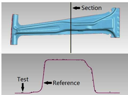
Figure 5: Springback minus maximum section.
