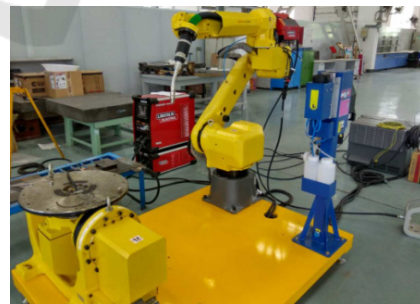
Figure 1. Robotic arc welding system.
