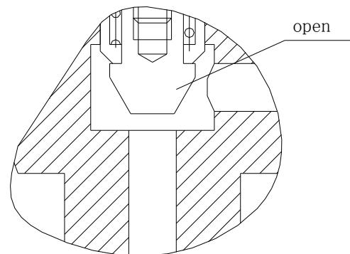
Figure 5: The diagram of electric valve open state.
