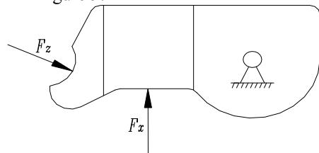
Figure 9: Force analysis of pressure arm.
