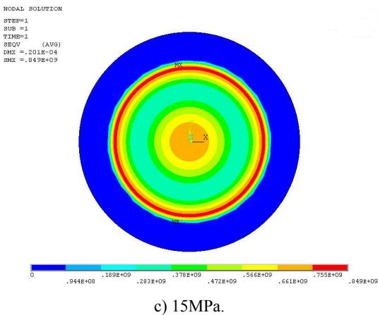
Figure 13: Pressure distribution under different pressure of the safety diaphragm.
