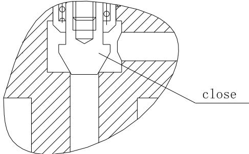
Figure 4: The diagram of electric valve closed state.
