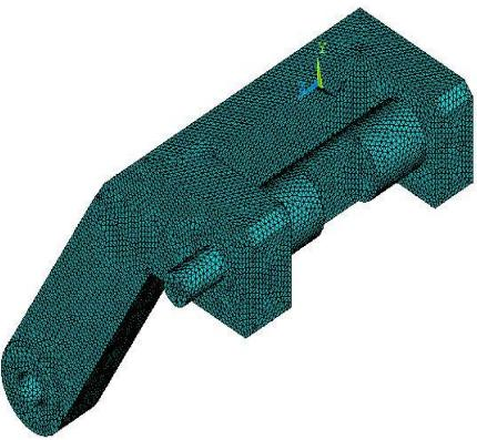
Figure 11: Finite element model of crank and shaft.
