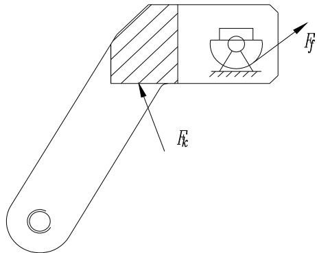
Figure 10: Force analysis of the axis and crank.
