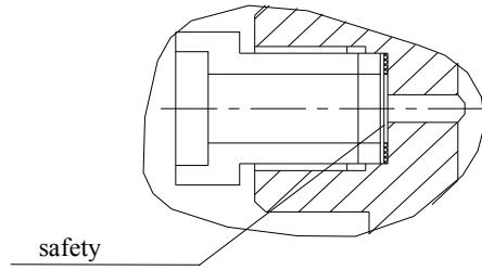
Figure 3: The diagram of over pressure exhaust structure.
