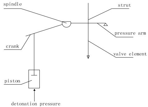
Figure 2: The schematic diagram of electric valve device.
