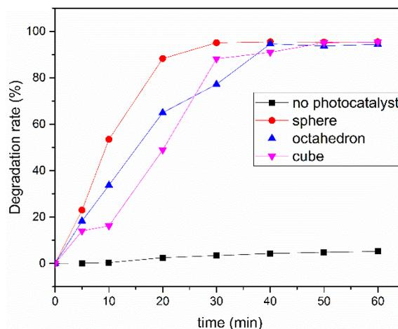
Figure 4:Catalytic degradation of MB curves byCu<sub>2</sub>O.
