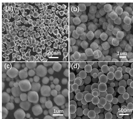
Figure 1: SEM images of the Cu<sub>2</sub>O samples with different morphologies.
