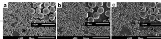
Figure 5: SEM images of 10wt% PCL in AA : EtOH = 8 : 2, at nozzle to substrate distance a) 24 cm, b) 20 cm, c) 15 cm, feed rate 0.2 μL/min, temperature 21°C, humidity 50%.
