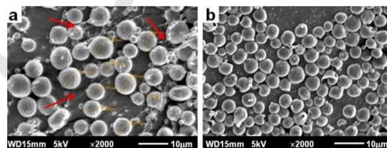
Figure 1: SEM images a) of 10 wt% PCL in AA, b) of 10wt% PCL in AA : EtOH = 8 : 2, temperature 21 °C, humidity 50%. Red arrow was eye guide for tiny fibres.
