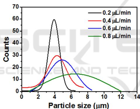
Figure 4: Gaussian fitted curves of size distribution histograms of 100 PCL particles at different feed rate.
