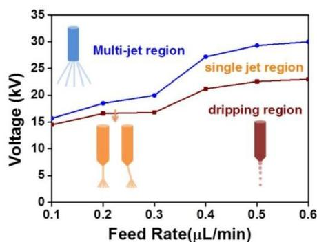
Figure 2: Critical voltage as a function of feed rate and spray mode classification according to the jetting: dripping region below the wine line, single jet region between wine and blue line, and multi-jet region above the blue line. The polymer concentration was 10wt% in mixed solvent AA : EtOH = 8 : 2, nozzle to substrate distance 20 cm, temperature 21°C, humidity 50%.
