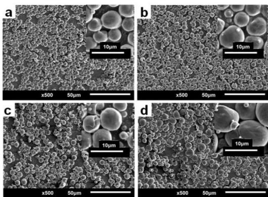
Figure 3: SEM images of 10wt% PCL in AA : EtOH = 8 : 2, at feed rate a) 0.2 μL/min, b) 0.4 μL/min, c) 0.6 μL/min, d) 0.8 μL/min, distance 24 cm, temperature 20 °C, humidity 50%.
