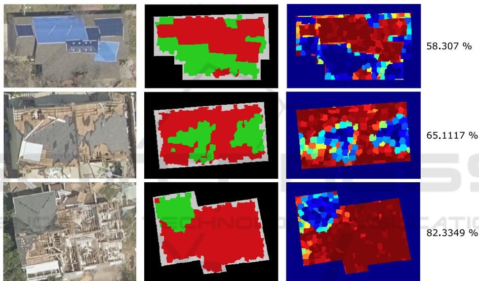
Figure 4: Selected results for D1: (left) orthophoto, (middle) locations of damage, and (right) probability map and damage grading. Dark red indicates regions that are most likely damaged while dark blue indicates regions that are most likely undamaged. The proportion of damaged roof area is given by the percentage values to the right.
