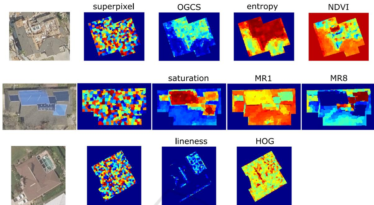
Figure 1: Alarm rates of selected features shown for three exemplary buildings. The first seven feature images clearly delineate the damaged parts of the roof from undamaged areas. The lineness and HOG reliably indicate the positions of roof edges and the texture salience.
