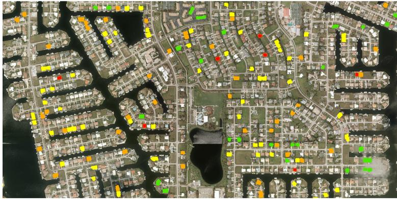
Figure 3: Visualization of damaged buildings on a map. Buildings in the portfolio are colored according to the damage ratio (green: intact, yellow: light damage, orange: medium damage, and red: heavy damage).
