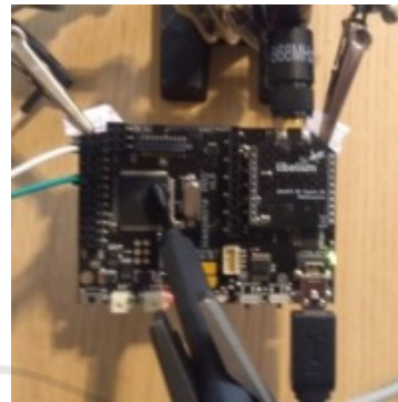
Figure 3: EM-leakage measurement from a end-device.
