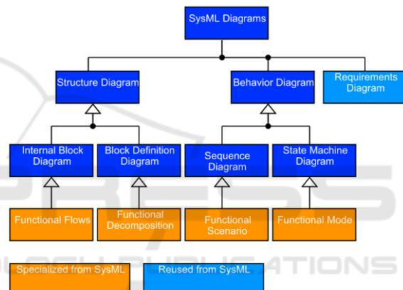
Figure 1: The set of diagrams used to model the functional view.
