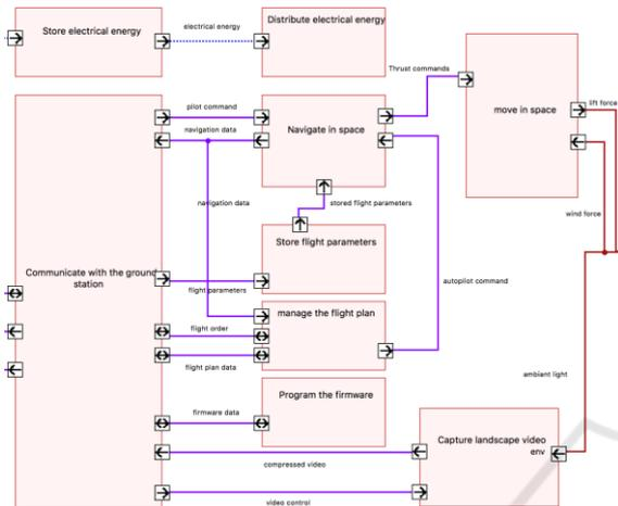
Figure 2: Abstract of functional flow diagram from the quadcopter model.
