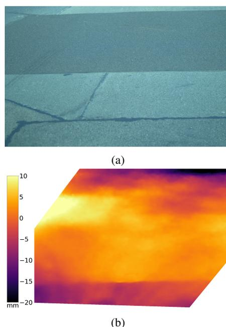
Figure 5: (a) Right image, captured from behind the windshield of a moving car at  $75\text{kmh}^{-1}$  and (b) corresponding depth map created with the CNN method.
