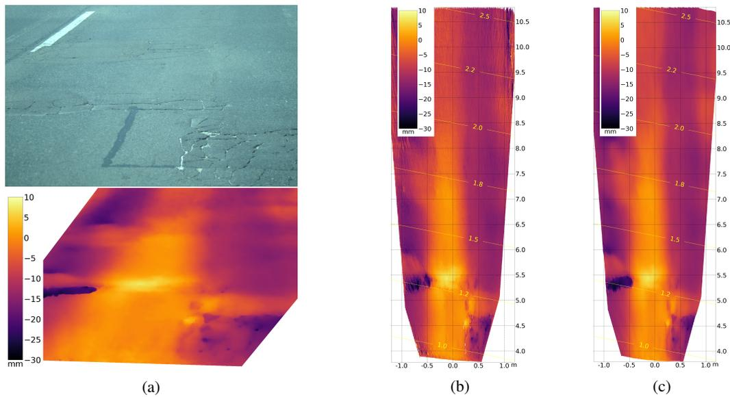
Figure 3: (a) Right image, captured from behind the windshield of a moving car at  $37 \text{ km h}^{-1}$  and corresponding depth map created with CNN method, (b) depth map from a bird's-eye view with contour lines, indicating depth resolution in mm/pixel created by SGM method and (c) created by CNN method.
