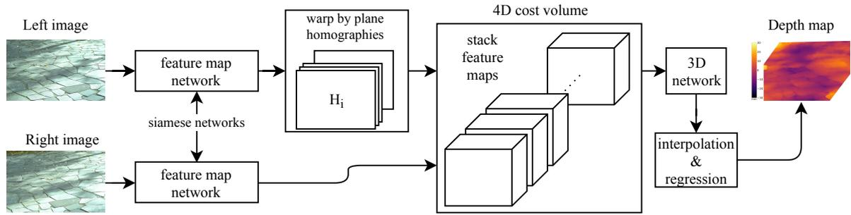
Figure 1: Feature maps are calculated by a Siamese network for both input images. One of them is transformed by a plane homography and a 4D cost volume is created. Matching is done by the 3D network, which outputs the depth map.
