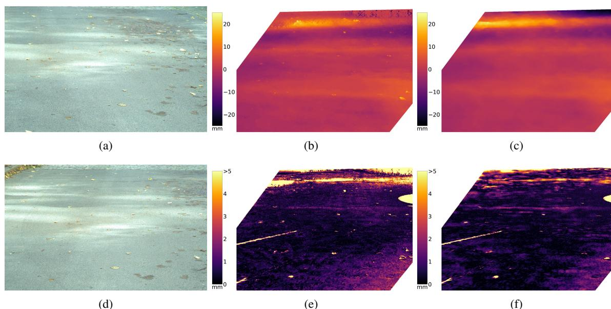
Figure 2: Static scene: **a,d** left and right image **b,c** depth map generated by SGM and CNN method (viewed from the right camera perspective) **e,f** error between laser scan reference and SGM/CNN method. The circular part on the right and the stripe on the left are artefacts of the laser scan. The distance between camera and the lower part of the image is 4.5 m, between camera and upper part 13.0 m.
