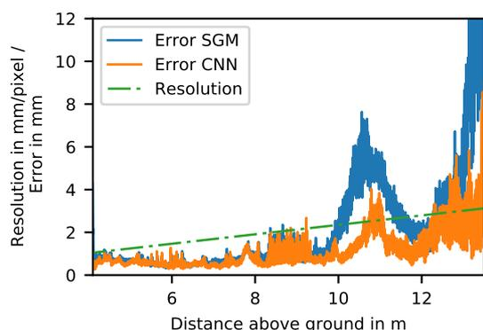
Figure 4: Errors of the SGM and CNN methods compared to the laser scan are shown, which increase over distance from the cameras. The physical depth resolution of the stereo camera setup decreases over distance.
