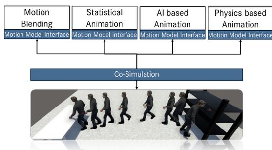
Figure 1: Principle of the Motion Model Unit approach. Using standardized units for encapsulating heterogeneous character animation approaches and a co-simulation, multiple systems can be incorporated into a common platform.
