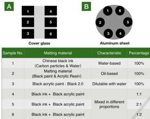
Figure 2: Configuration diagram of the matting material and substrate type.
