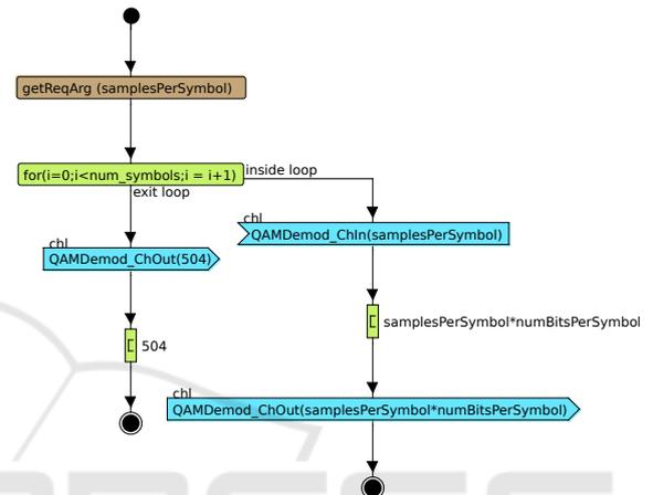
Figure 8: The UML AD for the data-processing part of an operation (X\_QAMDemod) for the centrally controlled view.
