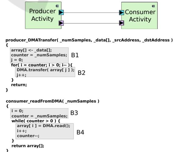
Figure 2: The SysML BD for a pair of Activities (upper part) and the pseudo-code of the Ports' ProtocolStateMachines for a DMA transfer (lower part).
