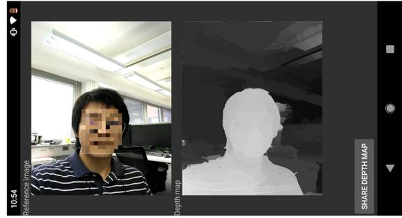
Figure 4: Depth-map demo on "selfie" sequence for ANDROID mobile device using CPU-GPU optimized co-processing.
