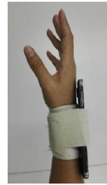
Figure 2: Smartphone attached to the wrist with a wristband.
