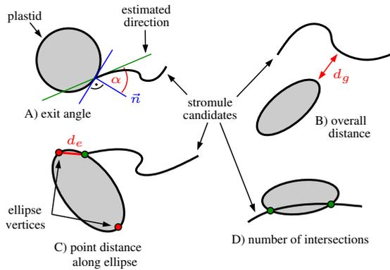
Figure 3: Geometric criteria to filter stromule candidates: they need to emanate from the surface almost perpendicular (A) and be located close to the plastid (B). In case of elliptical plastid regions they tend to start off close to the ellipse vertices (C) and usually do not cut through a region (D).
