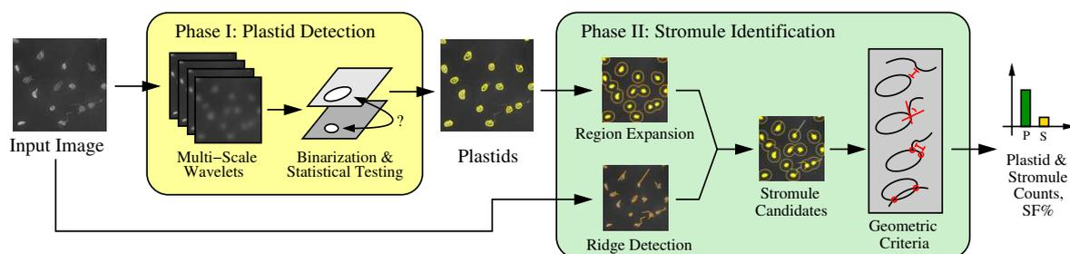
Figure 2: Overview of our approach: in the first phase (yellow box) plastid regions are extracted from input images, in the second phase (green box) curvilinear segments are detected in the vicinity of each plastid region and various geometric criteria are applied to classify them as referring to a stromule or originating from image artefacts and distracting signals.
