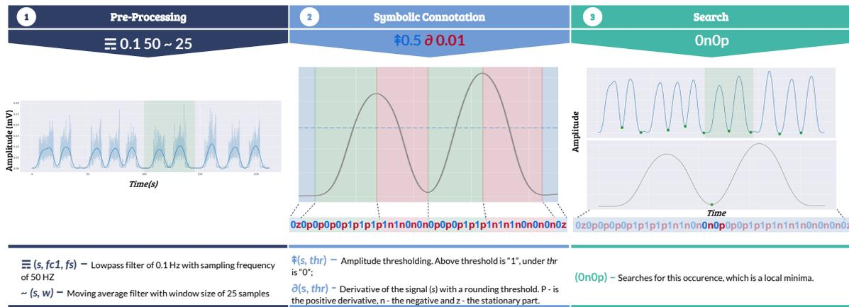
Figure 3: Initial sEMG segmentation. The sEMG signal is divided into cycles, which give an initial estimation of the activation period. Cycles are calculated by finding local minima using Syntactic Search for Time Series (SSTS).
