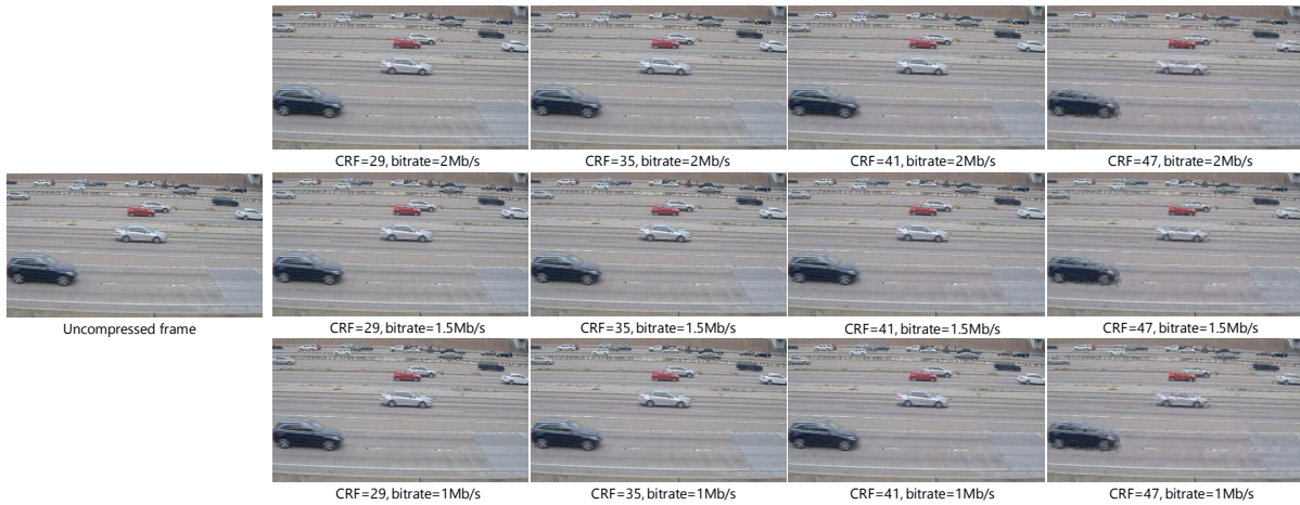
Figure 3: An uncompressed video frame and its 12 compressed versions. The compression artifacts can be visually perceived as CRF value increases and bitrate decreases. The combination CRF=29 and maximum bitrate of 2Mb/s results in lower compression, thus better video quality. The combination CRF=47 and maximum bitrate of 1Mb/s results in higher compression, thus worst video quality.
