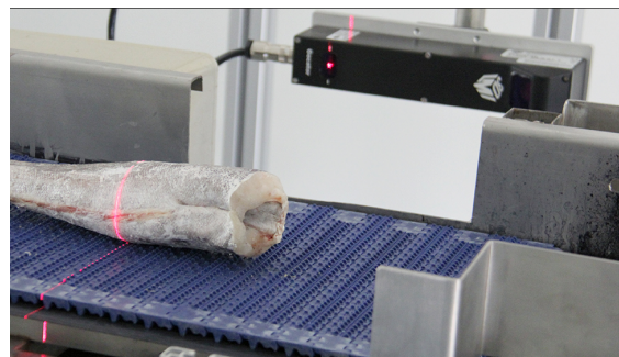
Figure 1: Hardware prototype of the acquisition module, including sensors that emits and capture lines of laser that are projected in the fish body over the conveyor belt.
