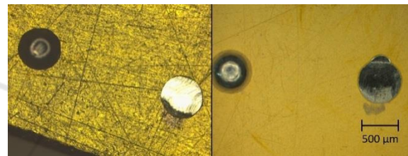
Figure 13: The shear test (before and after) on KOVAR Ni-Ti/Pt/Au and KOVAR Ni-Au.
