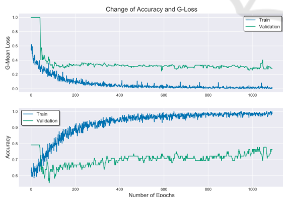
Figure 2: The average batch-wise G-mean loss and accuracy of the deep neural network as it is trained.
