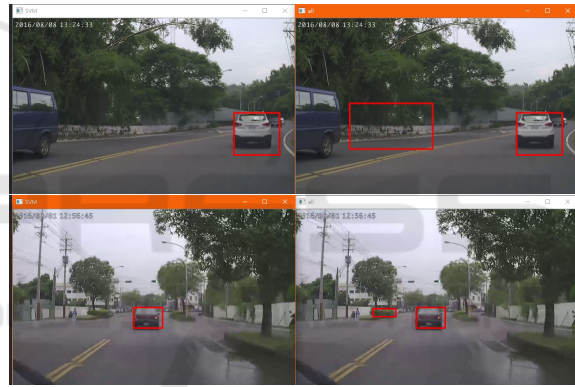
Figure 5: The results from HOG+SVM. The right and left images show the results before and after the verification mechanism is adopted.
