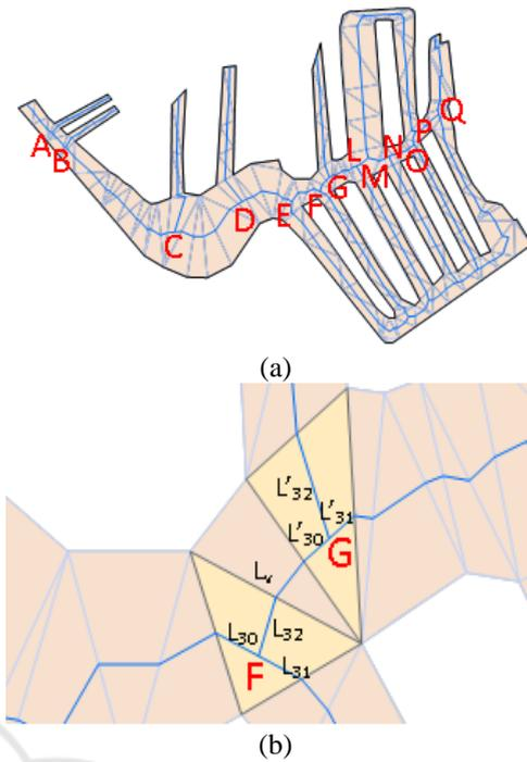
Figure 3: Trident association judgement. (a) Trident node, (b) Effective length  $L_v$  of connecting arc.
