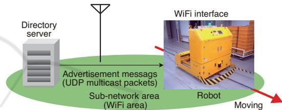
Figure 4: Communication between transport robot and directory server through WiFi.
