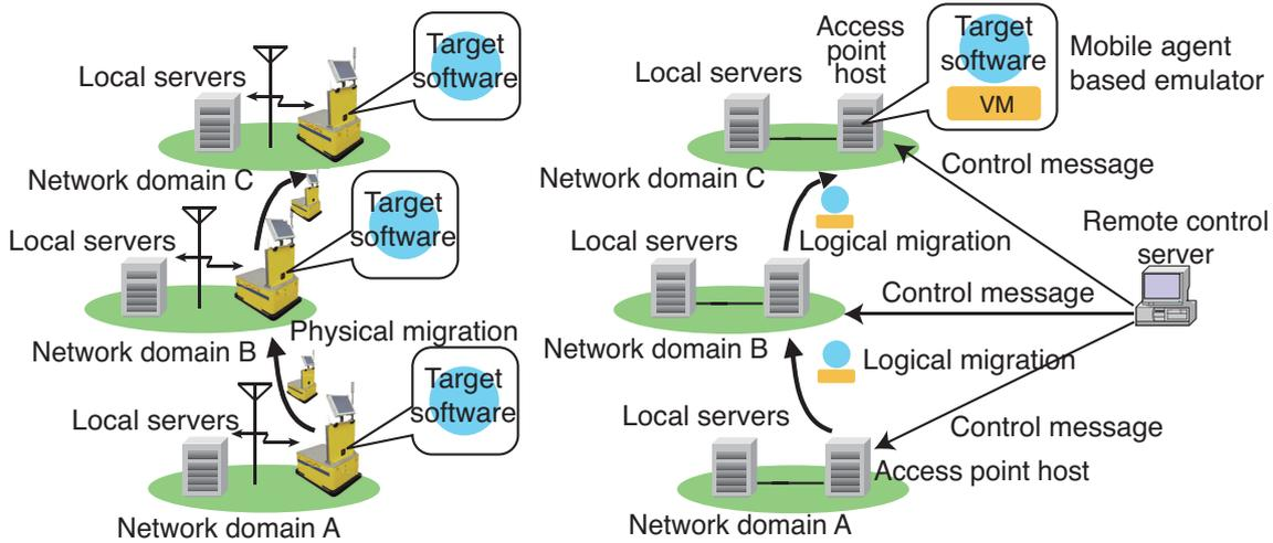
Figure 2: Physical mobility of robot (left) and logical mobility of emulator (right).
