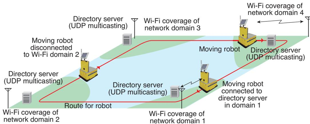
Figure 1: Transport robot with WiFi in a factory.
