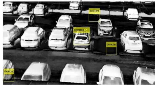
Figure 7: HOG based cascade detector.
