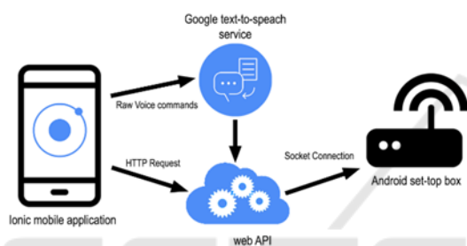
Figure 2: +TV4E mobile system architecture.
