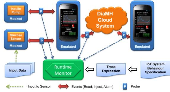
Figure 3: DiaMH Virtualization (Runtime Verification).
