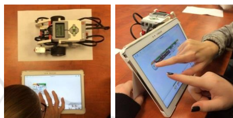
Figure 3: Programming of EV3 robot connected to the tablet via Bluetooth.
