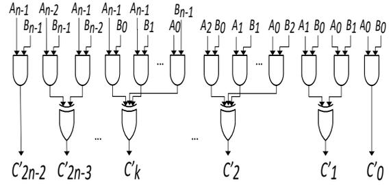
Figure 7: Logic Gate Implementation for the Classic Multiplier.
