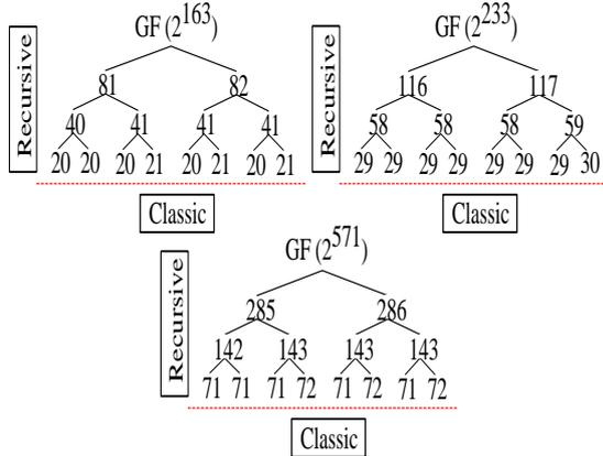
Figure 6: Recursive Splits over Different Finite Fields.
