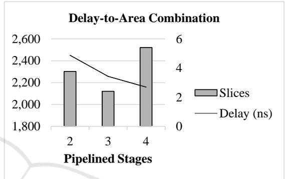
Figure 8: Delay-to-Area Ratio using Pipelined Stages.
