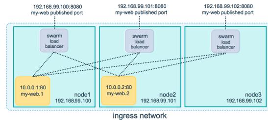
Figure 1: Docker routing mesh.
