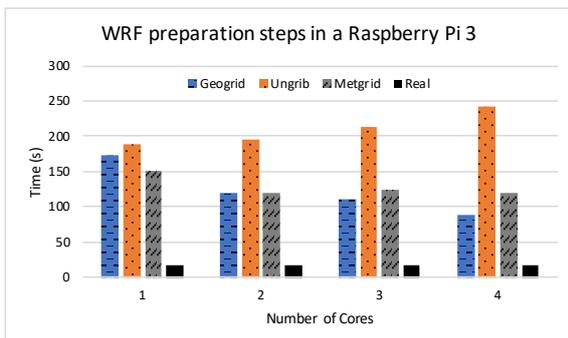
Figure 3: Performance of WPS steps when varying the number of cores.
