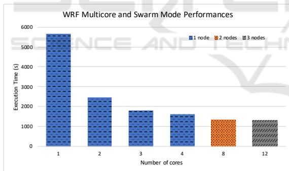
Figure 4: Performance of WRF in multicore and swarm cluster mode.
