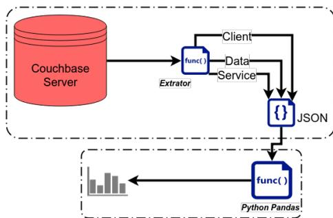
Figure 2: Extraction and analysis methodology.
