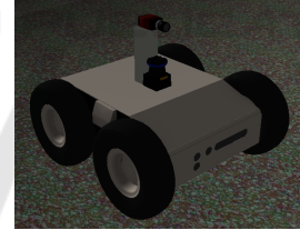
Figure 5: Dr Robot Jaguar equipped with a URG-30LX lidar and RGB camera.
