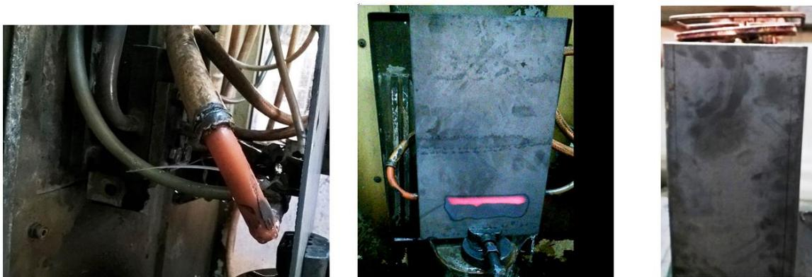
Figure 8: Experiments on induction hardening of the LGS profile's material.
