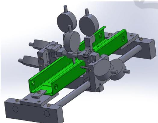
Figure 5: Control device for LGS profile.
