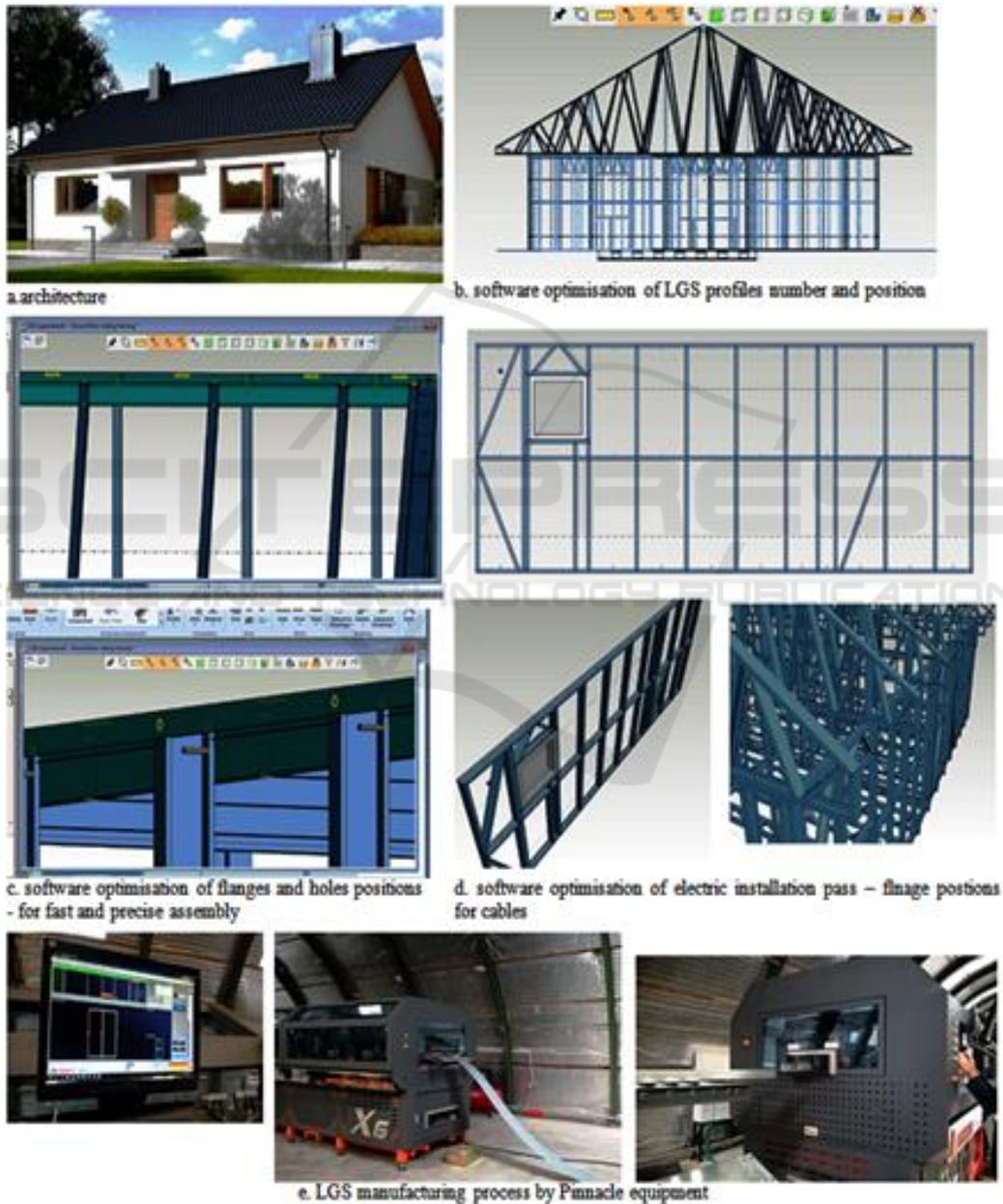
Figure 9: Intelligent manufacturing system.
