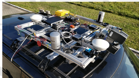
Figure 6: The Atlas sensory platform designed for surround sensing of autonomous vehicles. Line-Plane registration is used for mutual pose calibration of the FARO laser scanner and both Velodyne laser scanners.
