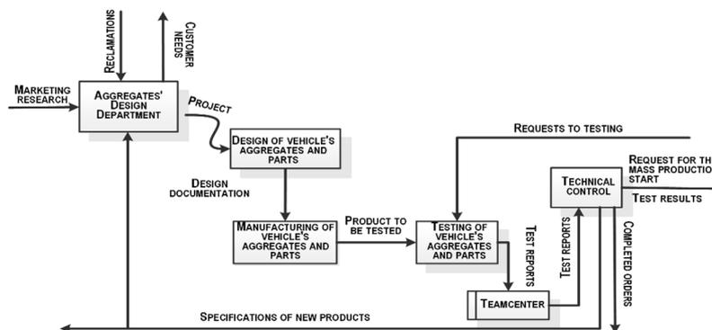
Figure 1: Data flows' processes diagrams of new vehicles models' designing, testing, starting mass production.
