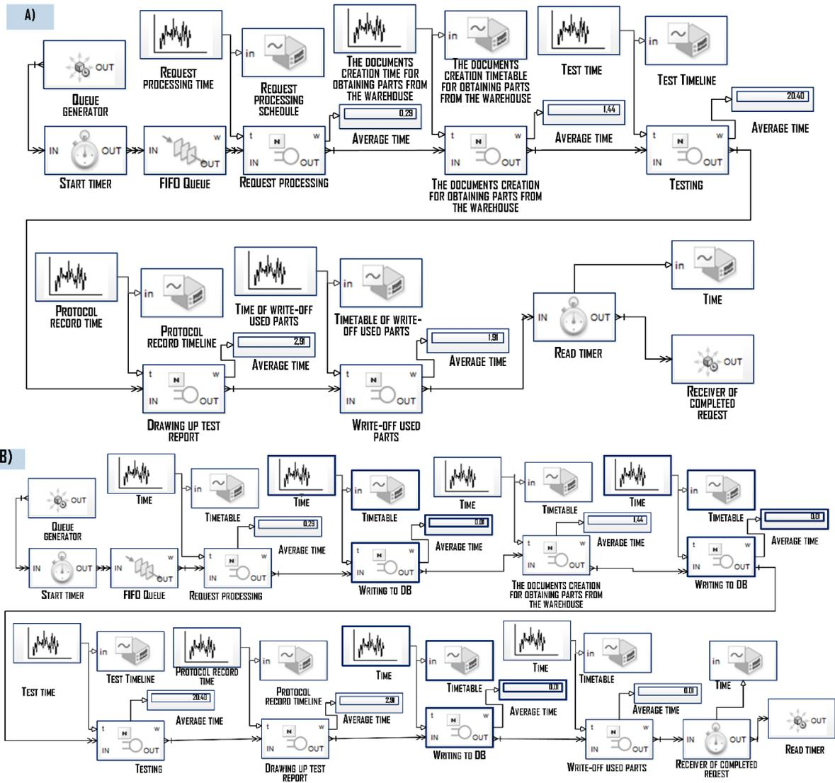
Figure 5: Process model a) before b) after DSS introduction (the record in the DB is distinguish with thick lines).
