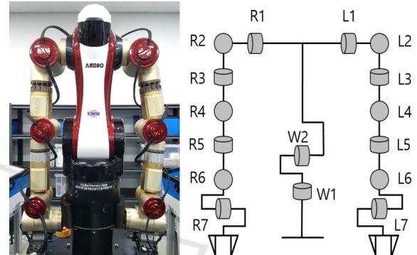
Figure 2: The developed industrial dual-arm robot, 'AMIRO'.
