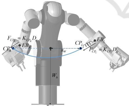
Figure 3: Conceptual view of the proposed method [front view]. Virtual springs are positioned between *CP* and elbows (*EB*).
