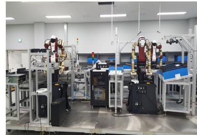
Figure 1: The developed robotic manufacturing system to pack cellular phones with multiple industrial dual-arm robots.
