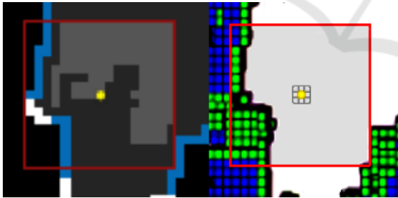
Figure 2: Algorithm 1 concept (2D view from above): robot (yellow) explores space behind contact space (red square area). Left image: fully explored contact space (white cells), partially explored contact space (blue cells) and free space (light grey) from which unexplored surface voxels are visible.
