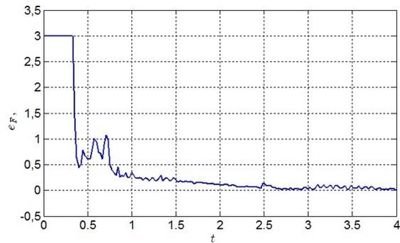
Figure 9: Transients of the force error for cylindrical object.
