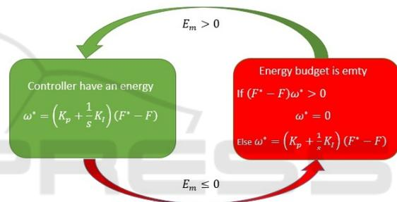
Figure 6: Finite state machine.
