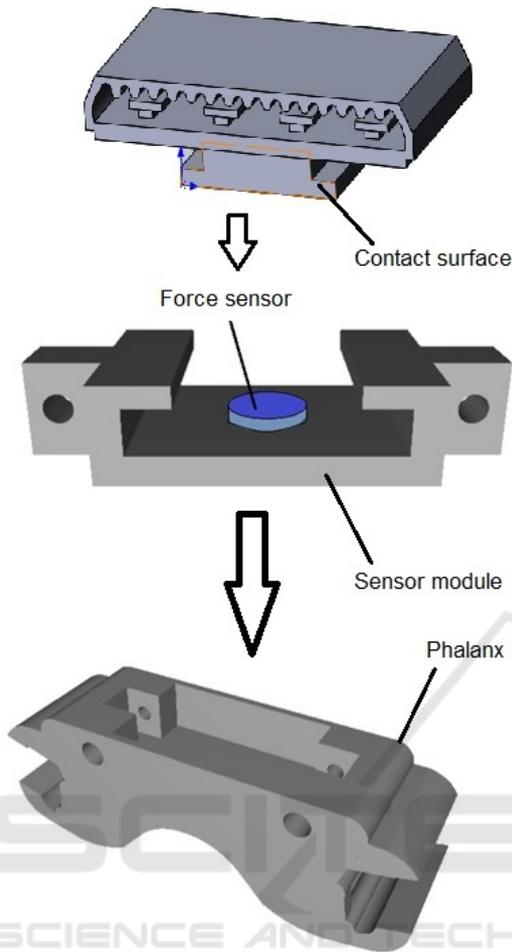
Figure 3: Sensor modular structure.
