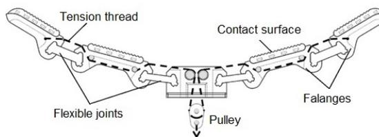
Figure 1: Differentially controlled pair of gripper fingers.
