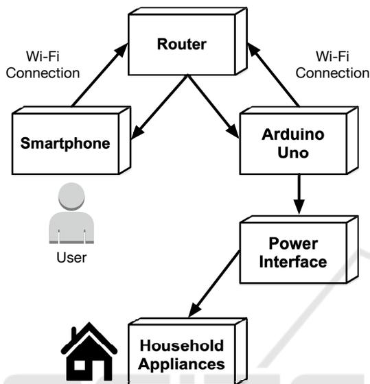
Figure 1: Block diagram of the domotic system - This figure shows the block diagram of the domotic system for people with disabilities. The smart phone can receive indoor location information from the Arduino located in each house area. It can also send on/off control signals to the household appliances.
