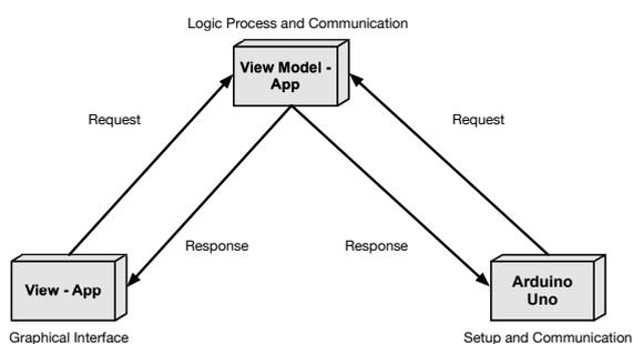
Figure 5: App graphical interface - This diagram shows the MVVM Model implemented in the development of software of the domotic system for people with disabilities. In the model layer the coding of the Arduino was implemented, in the view layer the code of the graphical interface of the APP was implemented and in the model layer the code necessary for the Wi-Fi connection processes of the system was implemented.
