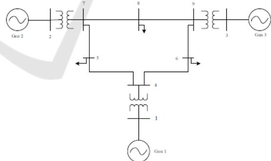
Figure 3: WECC 3-generator 9-bus test system.
