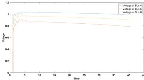
Figure 4: Plot of Voltages with Shunt block.
