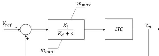
Figure 6: ULTC Block for Voltage Control.
