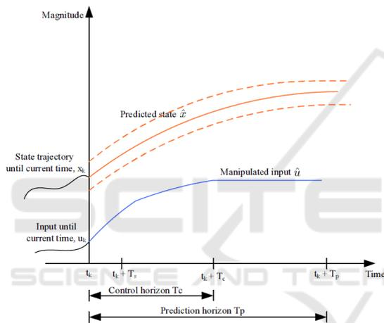
Figure 1: Principle of MPC.
