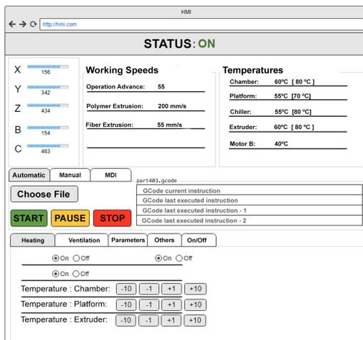
Figure 3: First static HMI prototype.
