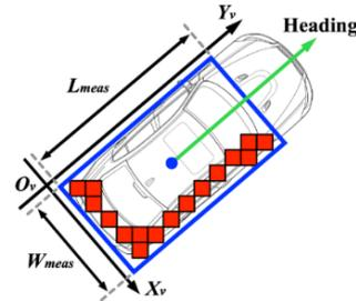
Figure 6: Observed vehicle size. Red squares and green arrow indicate moving cells and vehicle heading direction, respectively. Blue rectangle and circle indicate observed size and centroid, respectively.
