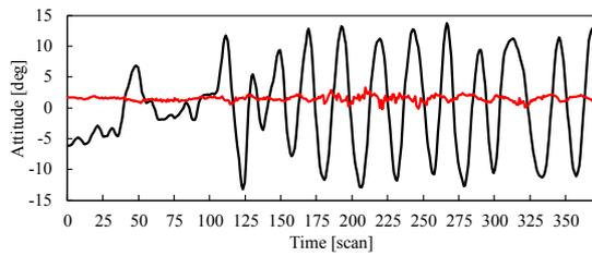
Figure 8: Attitude angles of bicycle. Black and red lines indicate the roll and pitch angles, respectively.
