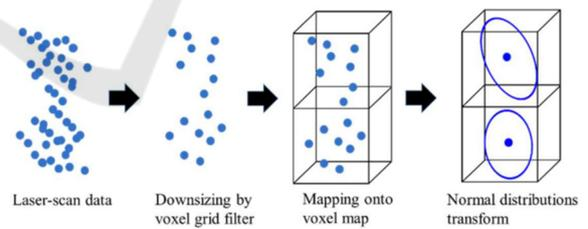
Figure 4: Mapping sequence of lidar-scan data.
