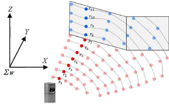
Figure 2: Extraction of lidar-scan data related to objects. Red and blue points indicate the scan data related to the road planes and objects, respectively.
