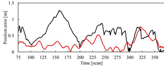
(b) Position error. Black and red lines indicate the error of the estimated positions in X and Y directions, respectively.
