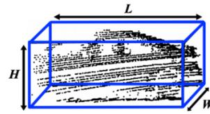
Figure 5: Cuboid around the tracked object (car).
