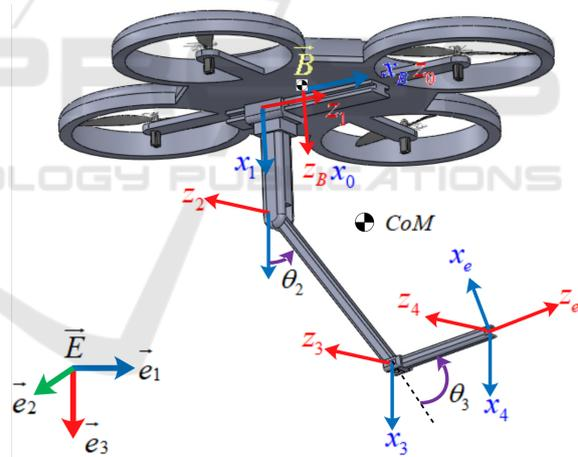
Figure 1: The structure of Q-PRR with principal frames.
