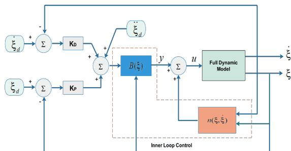
Figure 4: The control block diagram of Q-PRR.
