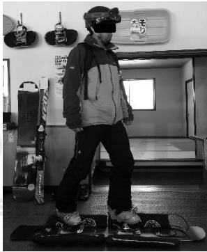
Figure 5: Snowboarder with attached measurement system.
