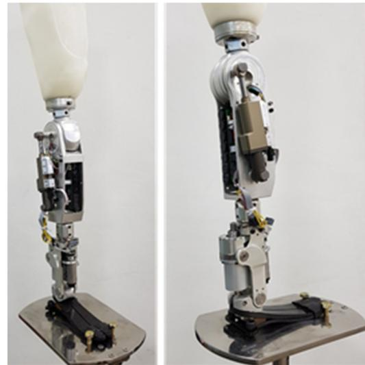
Figure 1: Hybrid above-knee prosthesis of KOREC.
