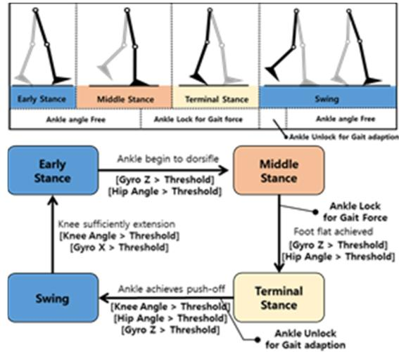
Figure 3: Control block of the ankle variable hybrid prosthesis.
