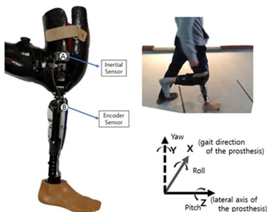
Figure 4: Passive type prosthesis adaptor and sensor attachment locations, experimental setting image and coordinate system used in this experiment.
