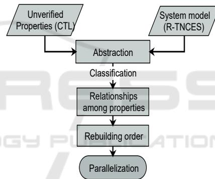
Figure 1: Parallel Rebuilding of R-TNCES.
