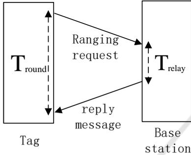
Figure 1: Schematic diagram of TOF distance measurement.
