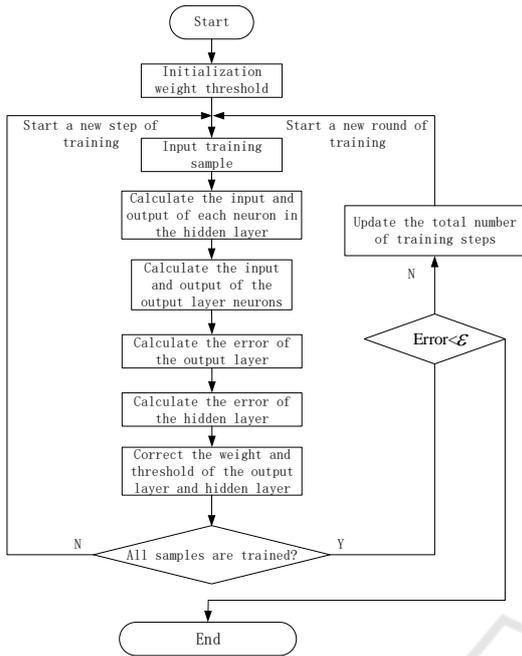
Figure 4: RBF algorithm flowchart.
