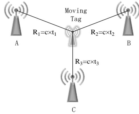
Figure 2: Principle of TOF positioning.
