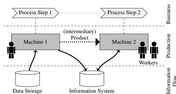
Figure 2: Running Example's simplified Industry 4.0 production context: different layers & perspectives.
