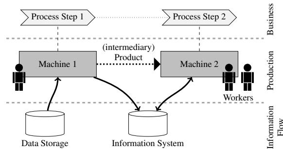
Figure 2: Running Example's simplified Industry 4.0 production context: different layers & perspectives.
