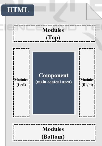
Figure 3: Template of a page in Joomla!-based Web applications.
