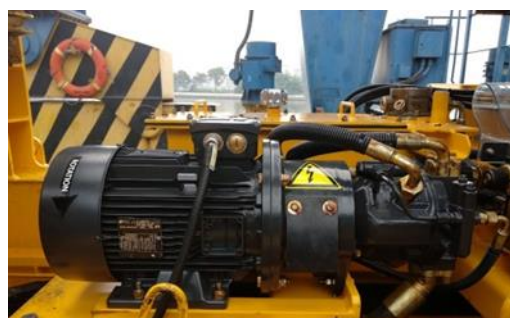
Figure 2: Three Phase Induction Motor on hydraulic pump Telescopic Spreader.
