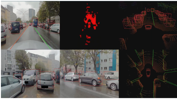
Figure 4: Results from LIDAR perception.
